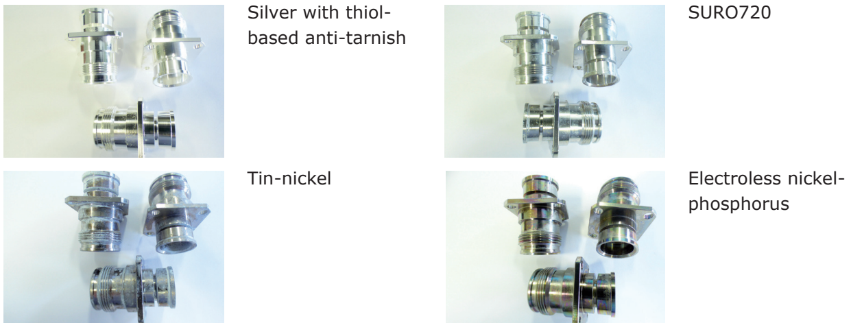
Figure 6 Corrosion of samples after 720 hrs salt mist test.
