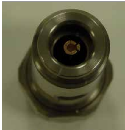
▲ Fig. 1 Adapter with a damaged finger.
